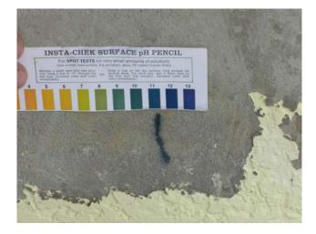
To test pH the most commonly used method is a pH pencil and distilled water. These pencils may be obtained from companies that distribute paint supplies. Most pH pencils are used by scratching a small area on the test wall and wetting it with distilled water. A color chart is provided to match the color of the test area with the corresponding pH color level.
